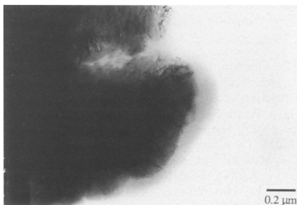
Figure 4 TEM micrograph showing the SiC-particle-PMMA interface.
